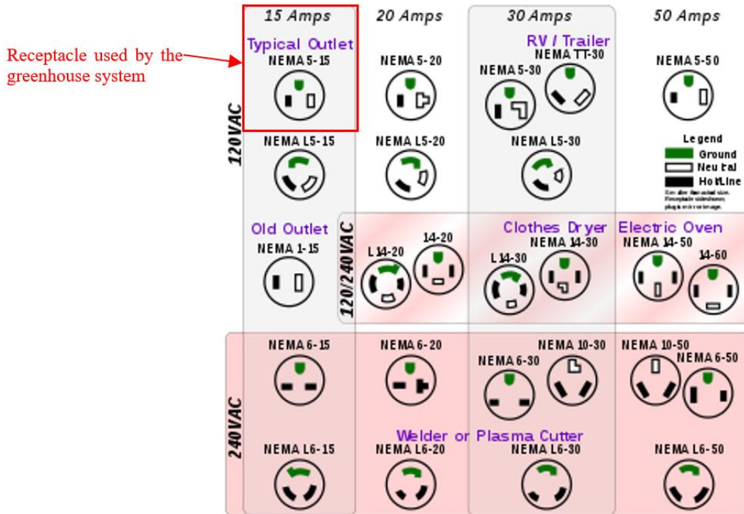
Figure 13- Receptacle and plug type used by the SmartLeaf system. Permissions requested from NEMAenclosures.com
